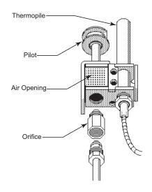
Figure 31. Honeywell Millivolt Pilot.
